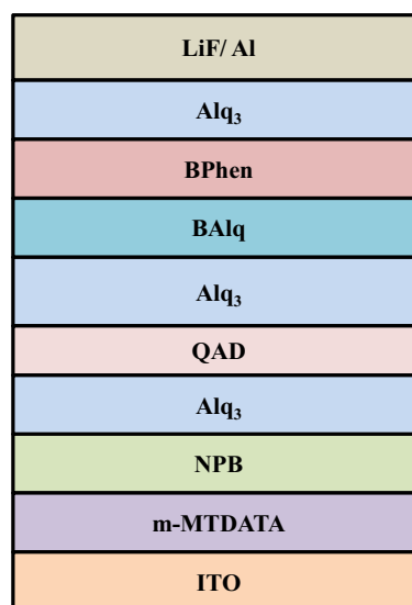
Fig. 7 Structure of double hole block layer OLED
